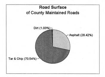
Of the 387 miles of County maintained roads, 110 miles are asphalt, 273 are tar and chip, and 4 miles are dirt.
